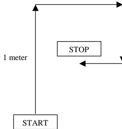
The visibly shortening length of each side reinforces the concept of a variable, the need for turning right the same way each time shows how constants are used, the successive nature of the required commands demonstrates sequential control flow, and the use of repeated subtasks to go forward and turn right illustrate procedures. The solution is available from the authors.
